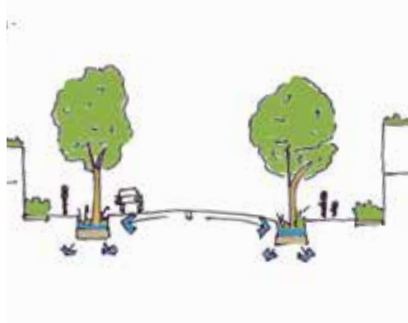
Street trees (with bioretention areas)
